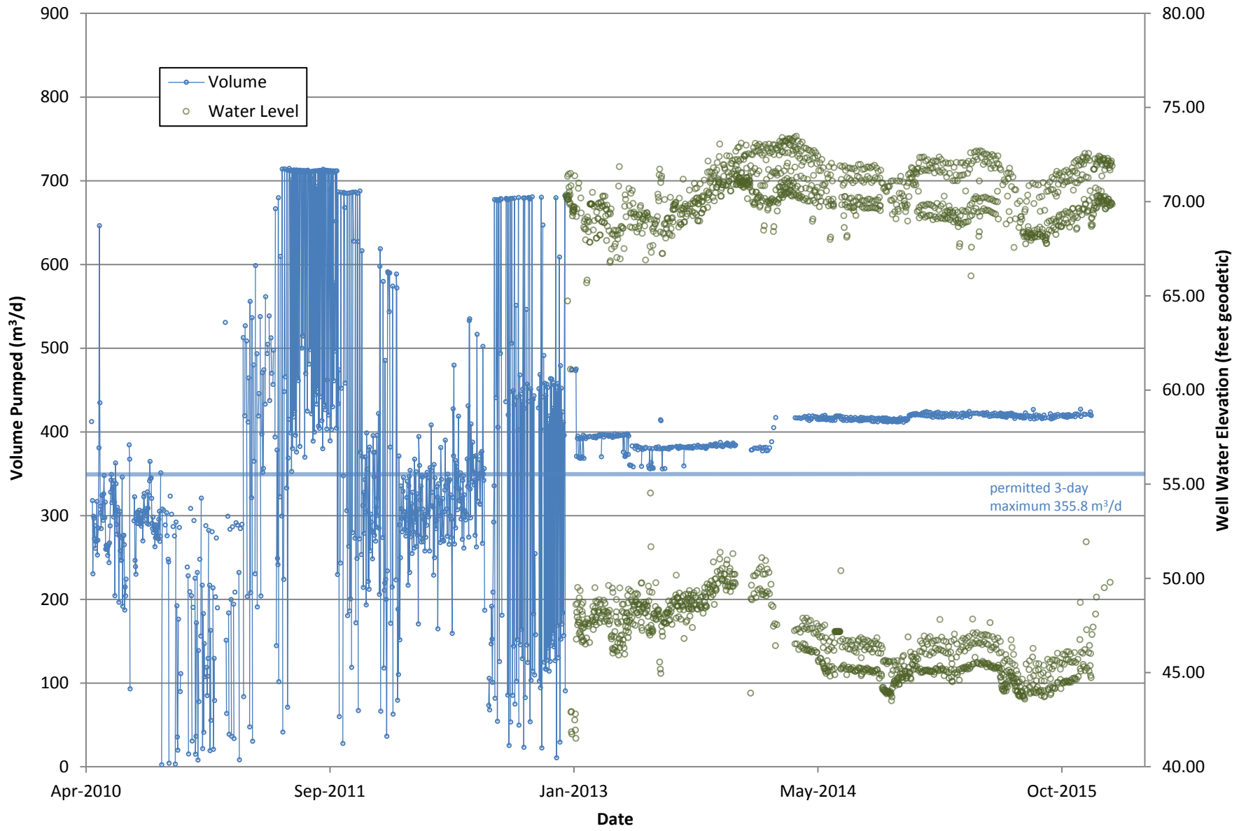
Figure 3.4: Daily Volume Pumped and Maximum and Minimum Water Levels in Production Well 3 (PW2)
