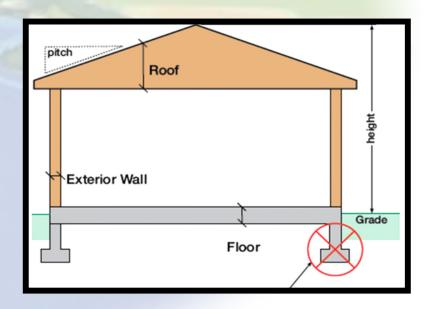
Note: A slab foundation is permitted provided the accessory building is less than 600 square feet in size.
